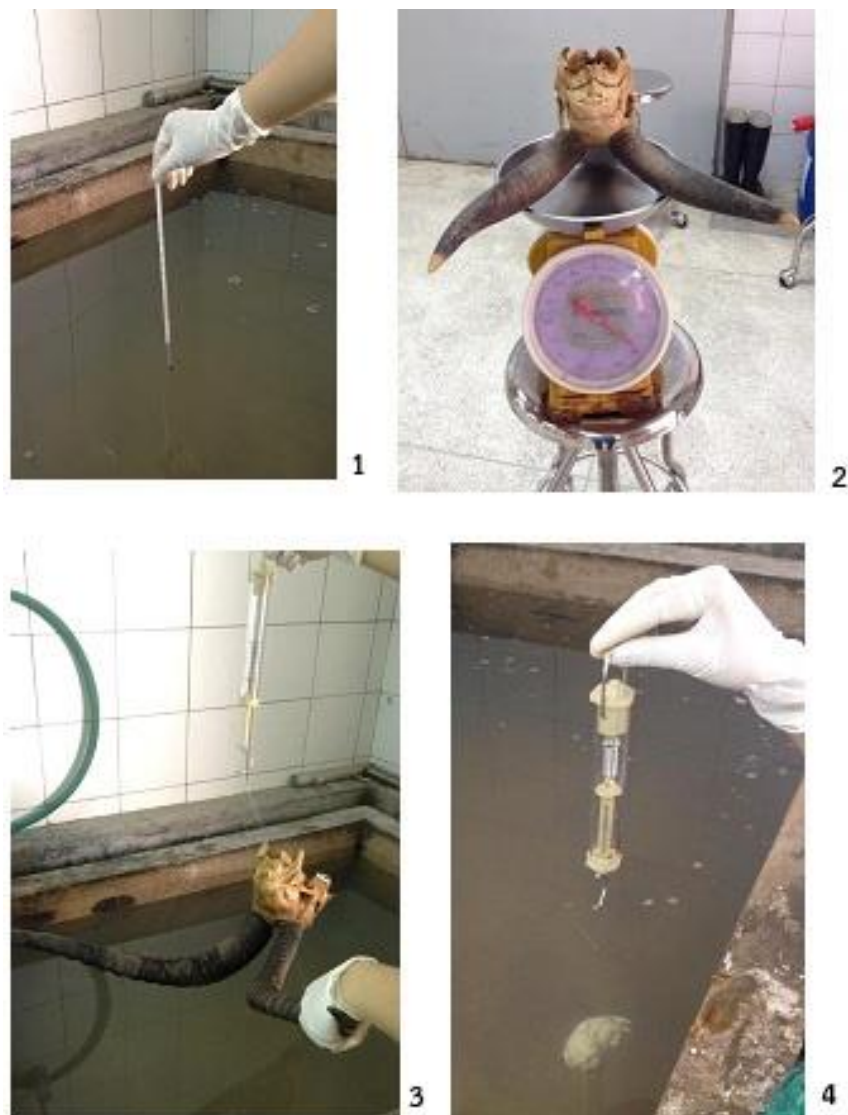
Figure 3 The skull volume morphometry. Measure water temperature (1) for density calculation. Weigh the skull (2). Next, suspend the skull on the scales then immerse the skull into water (3). Read the scales when the whole skull is fully immersed (4).
